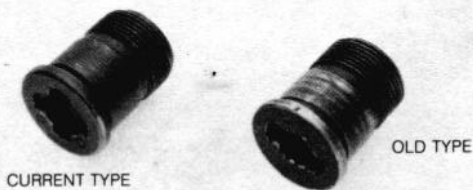
Figure 43. Gas cylinder cap screws, current type and old type.
